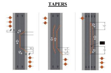
Tapers may be used in both the transition and termination areas. Whenever tapers are to be used near an interchange ramp, crossroads, curves, or other influencing factors, the length of the tapers may be adjusted.
