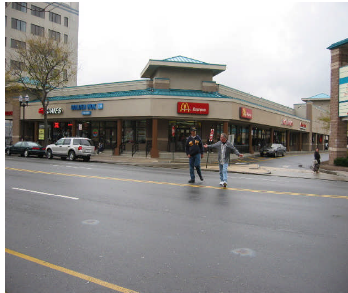
Undivided multi-lane arterials make shopping streets difficult for pedestrians; medians and curb extensions can help improve crossability.
