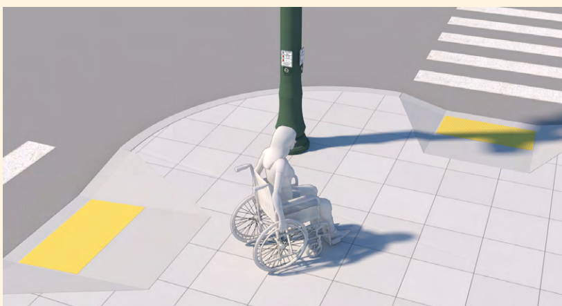
Curb ramps must be provided at all crosswalks. Ramps and pedestrian push buttons must be accessible to all users and meet the requirements of the Americans with Disabilities Act Accessibility Guidelines (ADAAG), which include standards on ramp width and slope.
