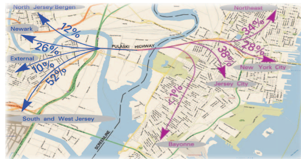
Map showing the distribution of vehicle trips via the Pulaski Skyway during the AM period. Blue lines indicate westbound destinations, while purple lines indicate eastbound destinations.
