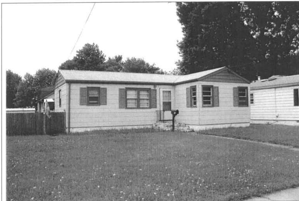
Photograph 2: 15 Roosevelt Avenue. Note the original door and windows, as well as the non-functional shutters. View looking west (May 2004).
