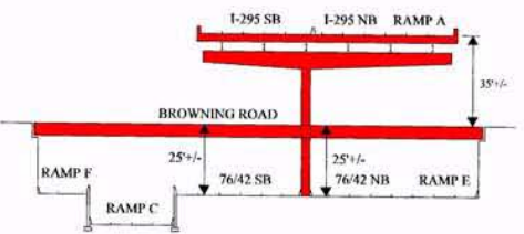
CROSS SECTION AT BROWNING ROAD LOOKING NORTH
