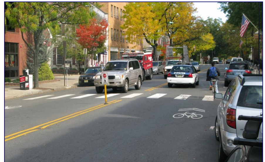
A network of Sharrow markings and enhanced crosswalks is recapturing Princeton's streets and creating a multimodal network that truly meets the goal of Complete Streets: serving all users and all modes on all streets.
