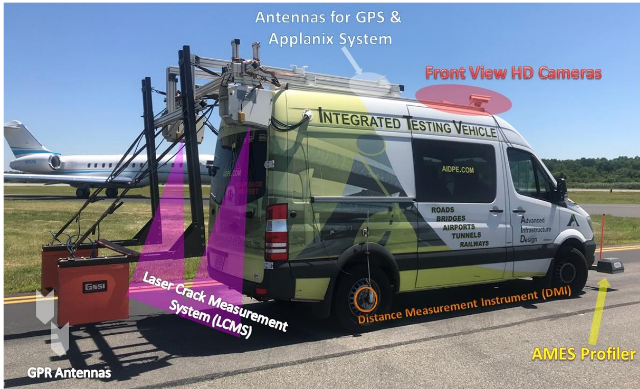
Figure 2. AID's Integrated Testing Vehicle (ITV)
