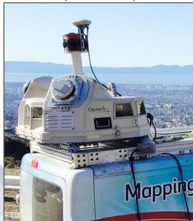
Figure 5. Mobile LiDAR system with spherical camera
