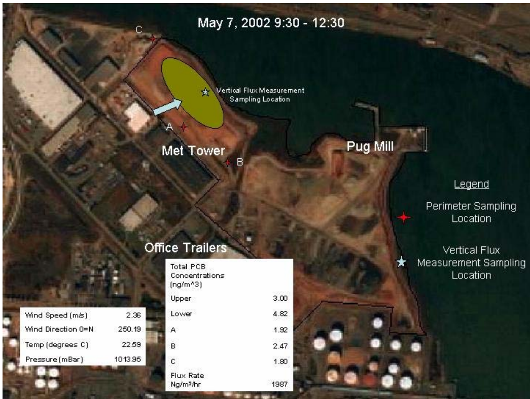
Figure 28. Bayonne landfill site conditions, 7 May 2002, 0930 – 1230 hours.
