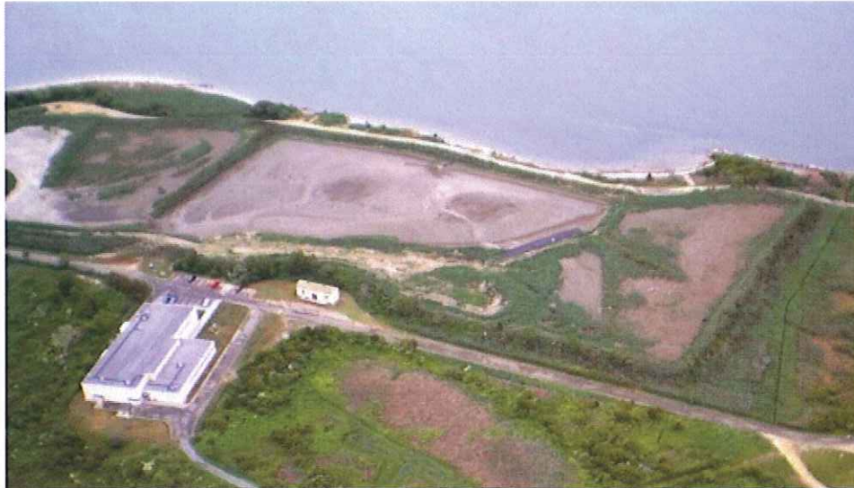
Figure 15. Site 3 after processing. The geotextile tube can be seen along the interior perimeter of the CDF.
