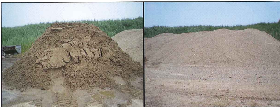
Figure 11. Stockpiled separated sand (left) and stockpiled recycled glass (right).
