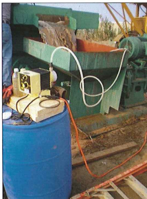
Figure 8. Polymer (blue drum), chemical feed pump, overflow basin and basin drainage pump
