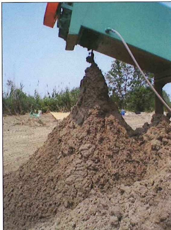
Figure 13. Processed sand being discharged from sand screw.
