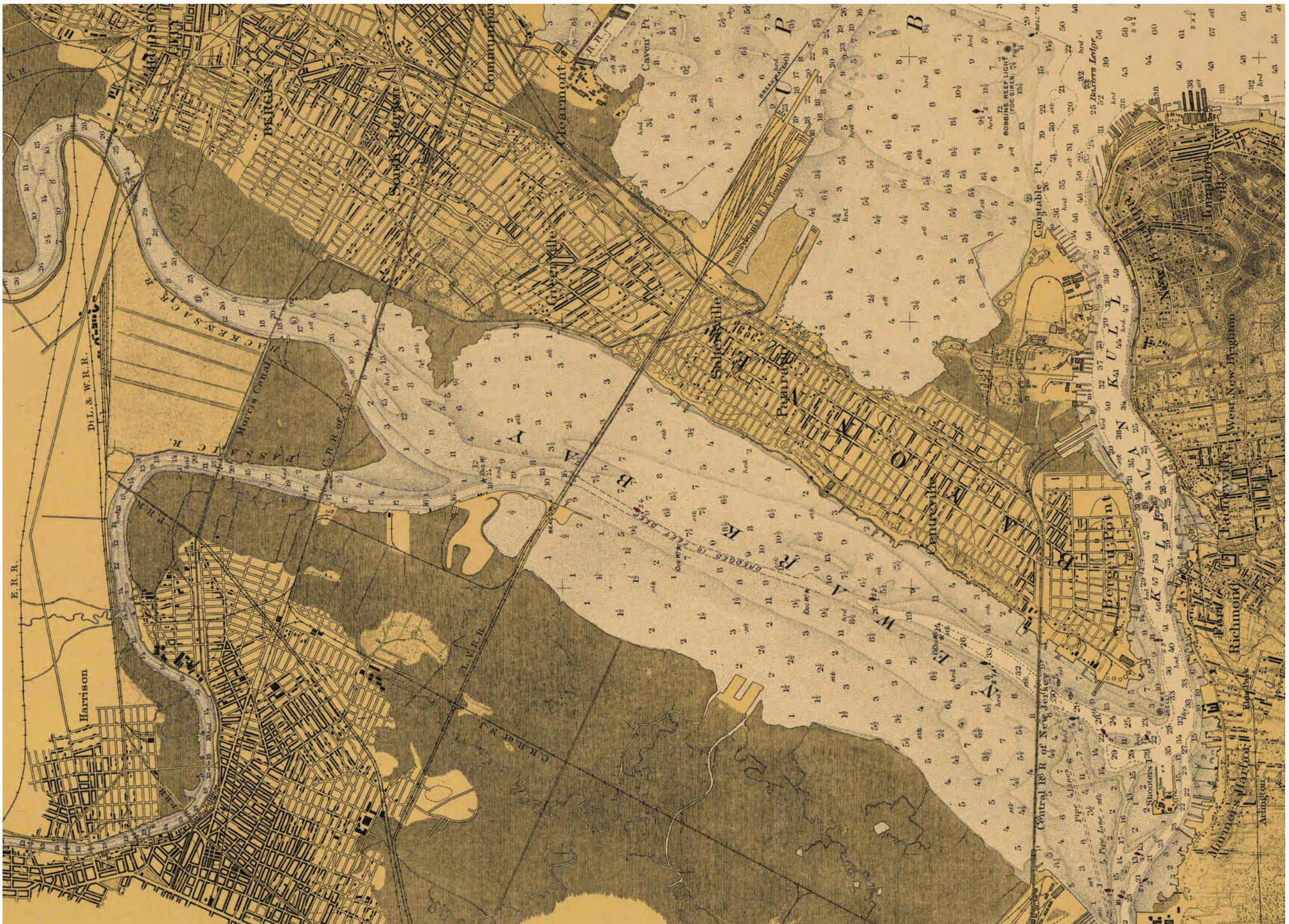
This 1914 coastal survey shows the recently dredged channel in Newark Bay and the depths of the Hackensack River (Coast and Geodetic Survey).
